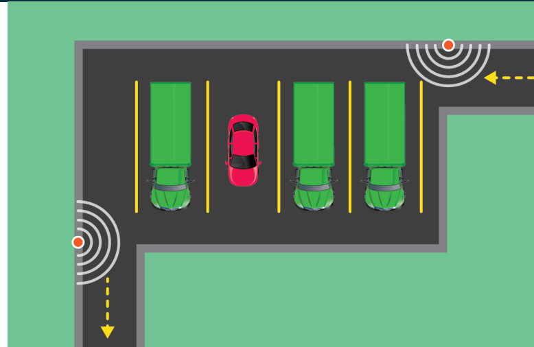
The system can also distinguish between commercial and passenger vehicles, allowing for notification of prohibited vehicles in designated parking areas.
