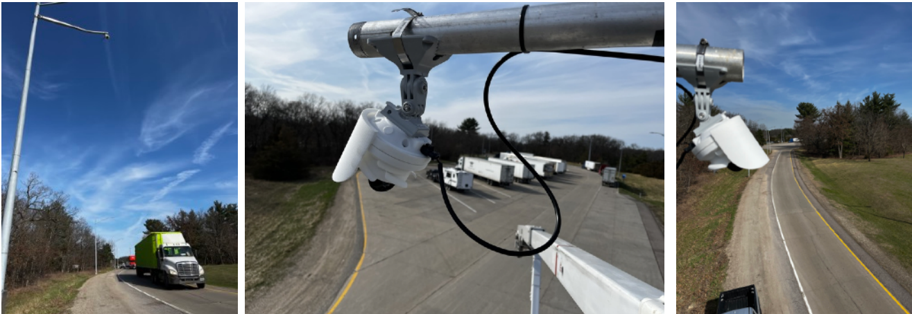
Example of HyPoint LiDAR-Based Monitoring System Installed for WisDOT at Rest Area 10
